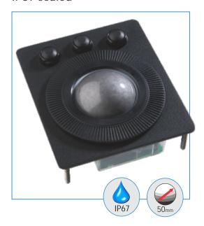
This unit consists of a 50mm infra-red optical trackball with removable ball and adjustable tracking force, with self-draining and flush through options and with three IP67 rated push button switches.
